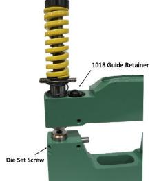
Extract the punch and apply a thin coat of lubricant (e.g. P/N 8007 Molykote® type G-N metal assembly paste) to the punch body. Put the punch and head assembly through a stripping spring (P/N 2045) and into the guide. Rotate the punch so the flat on the punch is parallel to the hole in the collar of the guide and push the retainer pin (P/N 2180) through the hole until it clips on to the guide collar.
