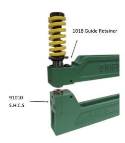
**Punch Installation:** First assemble a punch head (P/N 2171)
