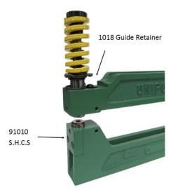
Then be sure the punch and head assembly will fit in the die by dropping it through the guide (without the stripping spring) and into the die. Visually look to see that the die clearance is even all the way around. If the die clearance is uneven, contact UniPunch.
