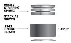
the bottom punch driver until tight. Insert punch screw thru top punch driver. Insert this top assembly into the top of the guide and screw into punch. Make sure to align the pin hole on punch with key slot on guide.
