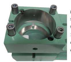
Assemble the (4) lifter springs (P/N 1470) into the four pockets on the upper arm of the holder. Then assembly the (4) spring cages (P/N 6043) on top of the lifter springs as shown in the picture on the left. Insert the (2) guide retainers (P/N 1018) into the two corner pockets of the upper arm of holder, making sure the flat on the guide retainer is facing the center of the guide bore of the holder.
