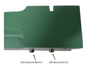
Using the same process as above, install the diamond pilot pin (P/N 1101) into the second hole making sure a point of the diamond shape faces the front of the unit.
