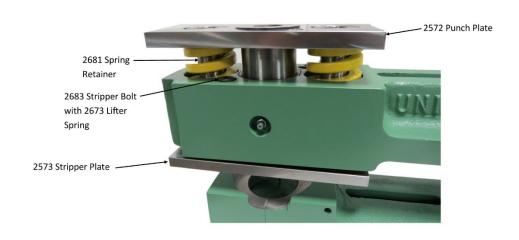
Assemble the (2) stripping springs (P/N 2540) into the two larger pockets on the top of the upper arm. Then put the punch plate (P/N 2572) on top of the springs and drop the (2) spring retainers (P/N 2681) down thru the center of the holes on the punch plate and down thru the center of the stripping springs. Then insert the (2) stripper bolts (P/N 2682) down thru the spring retainers and tighten into the stripper plate.
