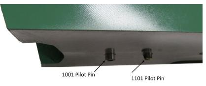
91332), supplied with pilot pin, until it touches the bottom of the hole, being careful not to push the pilot pin back out.
