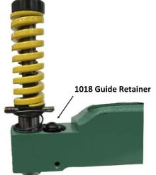
**Die and Die Adapter Removal:** To remove the round die (P/N 2120) from the die adapter, loosen the guide retainer (P/N 1018) on the top of the unit and lift the guide up. Loosen the set screw (P/N 91310 10-32 x .19 LG.) from the front corner of the die adapter and lift the die out of the adapter.
