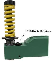
**Die and Die Adapter Removal:** To remove the round die (P/N 2120) from the die adapter, loosen the guide retainer (P/N 1018) on the top of the unit and lift the guide up. Loosen the set screw (P/N 91310 10-32 x .19 LG.) from the front corner of the die adapter and lift the die out of the adapter.
