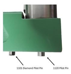
**Pedestal Die Removal:** To remove the shaped pedestal die (P/N 2126), first loosen the guide retainer (P/N 1018) on the upper arm of the unit to allow the guide to lift up. Use a hex key wrench to loosen and remove the 1120 pilot pin and lock washer from the lower arm of the unit and lift the pedestal die up and out of the unit.
