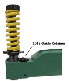
**Die and Die Adapter Removal:** To remove the round die (P/N 2220) from the die adapter, loosen the guide retainer (P/N 1018) on the top of the unit and lift the guide up. Loosen the set screw (P/N 91310 10-32 x .19 LG.) from the front corner of the die adapter and lift the die out of the adapter.
