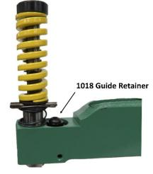
of the spring against the collar and insert the assembly into the guide bore while being sure to align the external key slot on the shaped guide with the dowel pin in the guide bore of the unit.
