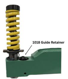
**Die and Die Adapter Removal:** To remove the round die (P/N 2320-1 or 2320-2) from the die adapter, loosen the guide retainer (P/N 1018) on the top of the unit and lift the guide up. Loosen the set screw (P/N 91310 10-32 x .19 LG.) from the front corner of the die adapter and lift the die out of the adapter.
