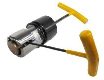
hole in the punch. Put the punch and guide assembly into a soft jaw vice and tighten the vice just enough to prevent the guide from spinning while you tighten the screw. Use a hex key wrench to tighten the punch screw. **Important**: tighten the punch screw until the punch driver is tight against the punch so that during punching operation the punch driver is what engages the punch and not the
