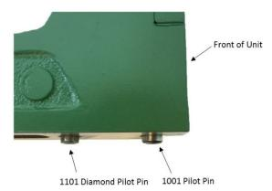
Using the same process as above, install the diamond pilot pin (P/N 1101) into the second hole making sure a point of the diamond shape faces the front of the unit.
