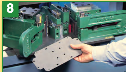
8 You can punch and notch multiple holes with each stroke of the press.
