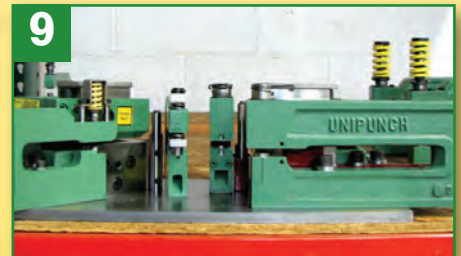
9 The tooling in the dedicated setup is assigned to the part for the life of the part. Here it is shown stored on a shelf, ready for the next time that part is required.
