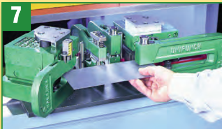
7 Depending on the application, material can be hand fed (as shown) or fed off a coil.
