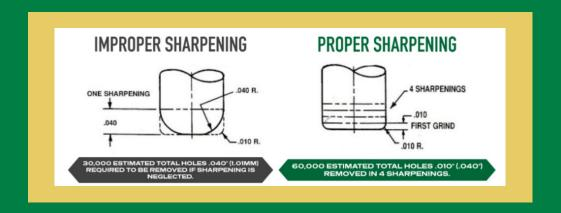
Tools not sharpened at the proper time demand additional pressure on the cutting edges which will deteriorate more and more rapidly. This in turn will decrease the hole quality and the quantity of holes that can be produced by that punch or die. Therefore, frequent sharpening is by far the least expensive way to produce consistent high quality holes.
