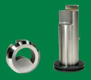
To insure proper line-up between the punch and die, the heel of the punch engages in the die prior to the punch cutting the material. The heel can also be used for part gauging.
